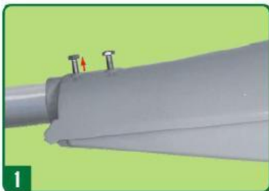
1 Unscrew the hex bolt M10×35. Fasten the fixture with the pole and tighten the bolt
